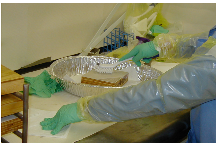
Figure 3-2. Laminate coupon being scrubbed with brush after DSG application.
