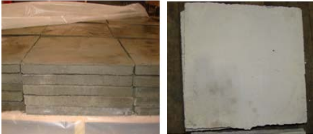
Figure 2-2. Curing Concrete (left) and Final Concrete Coupons (right)
