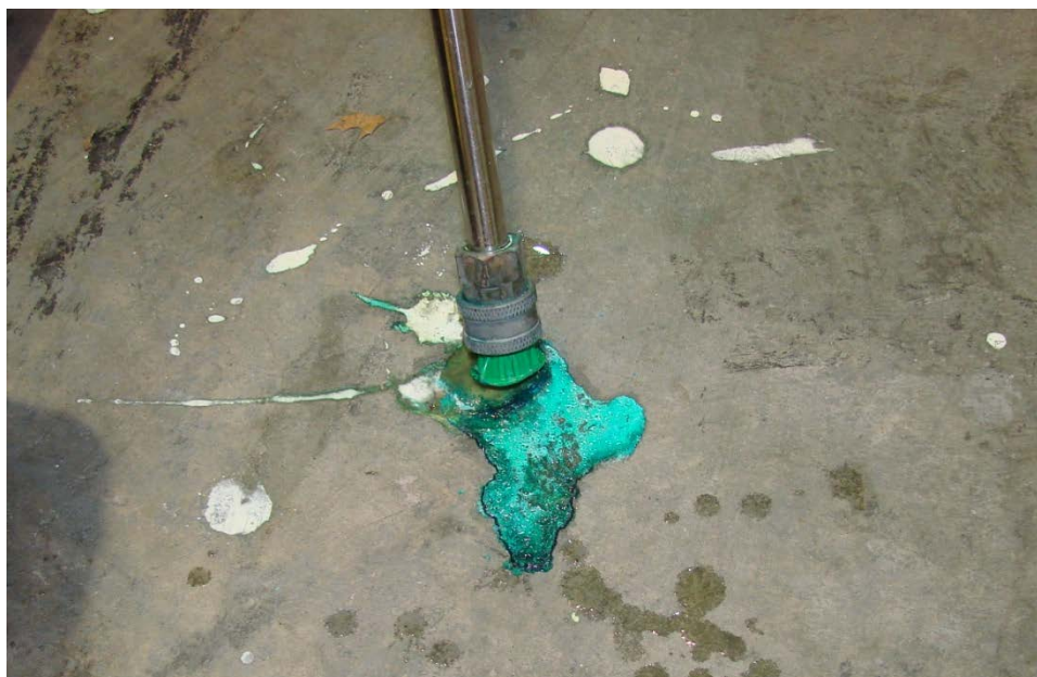
Figure 3-7. Corrosion on Pressure Washer Nozzle from Contact with Spor-Klenz®
