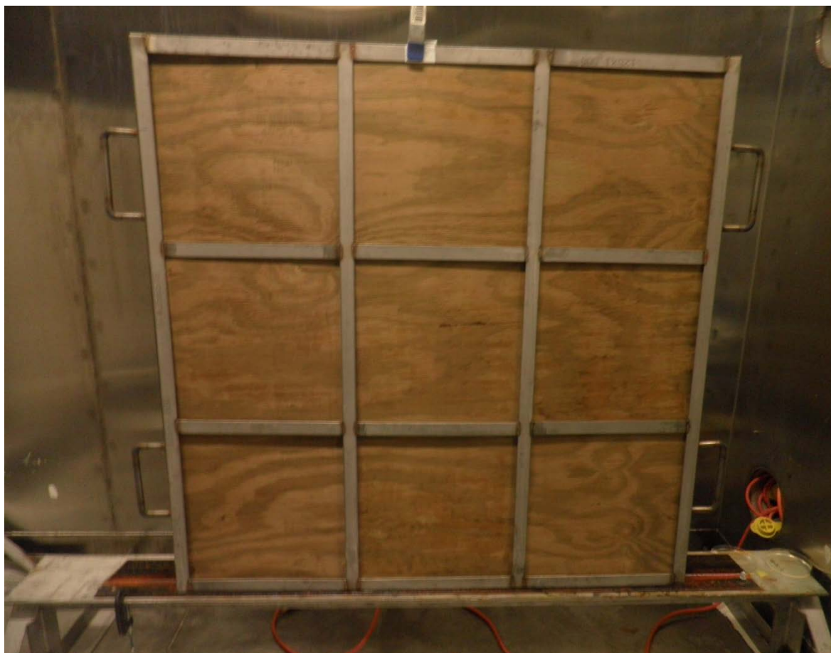
Figure 2-3. Sampling Template on Task II Pressure-treated Plywood Coupon
