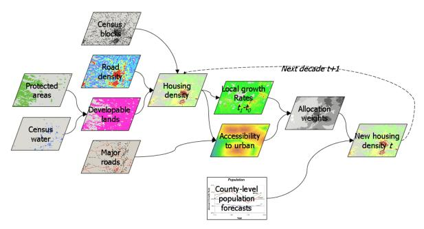
Figure 2-1. Diagram of SERGoM data inputs and modeling process
