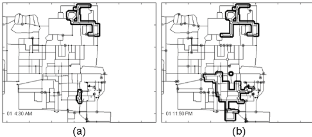
Figure 7-7. Scan test results for 100 sensing-nodes and two contaminant injections. (a) Results when both injections are first detected. (b) Results after 24 hours.
